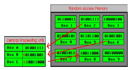
Any two bytes can be added from anywhere in RAM and the result placed anywhere in RAM.
