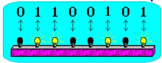
Most personal computers have at least 640k of Random Access Memory (RAM). Since a single k is 1,024, this means that these computers have (640 times 1,024 equals) 655,360 bytes of RAM. Since each byte has eight bits, this means that these computers have (8 times 655,360 equals) 5,242,880 bits in RAM.
