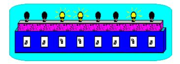
This is an imaginary and oversimplified concept of a primitive computer. However, early personal computers were similar to this. For example, they had switches to set individual bits. After the computing was finished, the user had to read and interpret lights which also represented individual bits.
